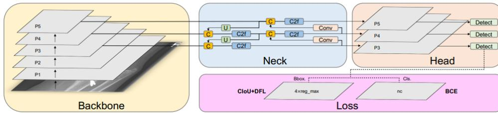
**Figure 2.** YOLOv8 architecture
