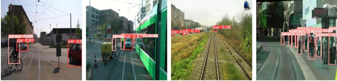
**Figure 3.** Test results of the YOLOv8m sub-architecture
