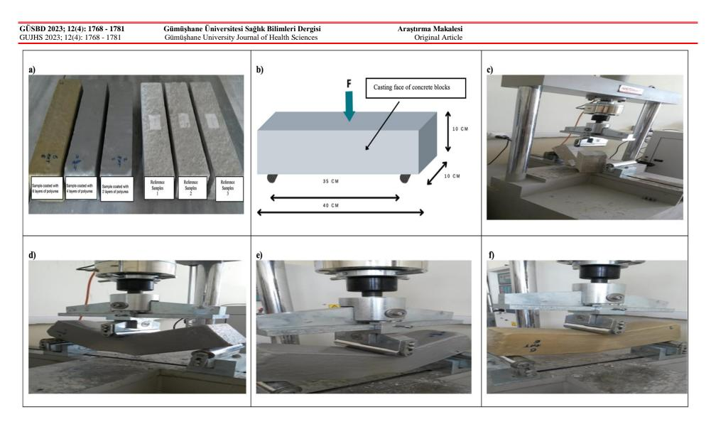
Figure 2. a) Polyurea-coated and uncoated (reference) concrete samples. b)3 Point Bending Testing apparatus. c) Brittle fracture in reference samples 1, 2, and 3 without deflection. d) Deflection in the sample coated with 2 layers of polyurea. e) Deflection in the sample coated with 4 layers of polyurea. f) Deflection in the sample coated with 6 layers of polyure
